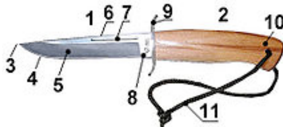
Fig. 63. (1) is the blade, (2) handle, (3) point of knife, (4) cutting edge, (5) grind, which is the cross section of the blade, (6) spine, which is the thickest part of the blade, (7) fuller, the groove which lightens the blade, (8) ricasso, barrier between the blade located at the junction of the blade and the knife's bolster or guard, (9) guard, the barrier between the blade and the handle, which protects the hand from an opponent, (10) the end of the handle or butt, and (11) the knife's handle or butt may allow a lanyard to be used to secure the knife to the wrist, or a portion of the tang to protrude as a striking surface for hitting or glass breaking.
